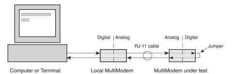
Figure C-4. Back-to-back test.
